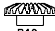
BA2 ×2 ベベルギヤ (大) Large bevel gear Kegelrad groß Grand pignon conique 51008
